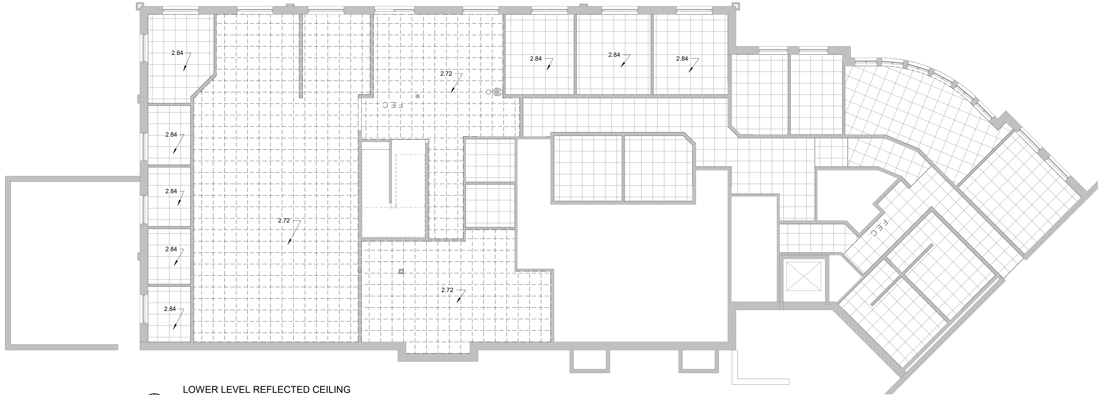
LOWER LEVEL REFLECTED CEILING DEMOLITION PLAN 1/8" = 1'-0"
